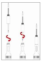
Insert the other end of the tube into the middle of the base while turning the front portion to tighten it into the base's thread, don't overtighten.
