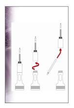
Unscrew the probe from the base of the device and slip the tube into the rubber holder in the front portion of the probe.
