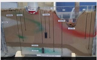
The groundwater hydrology model – the green and red colours are from dyes added to the water to track the way it moves underground.
