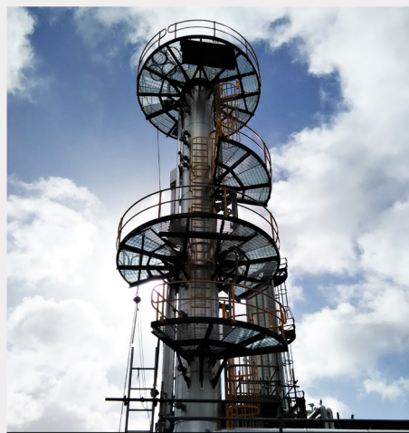
The new KPS stabiliser which is expected to reduce emissions by at least 4,500 tCO 2 e per year.
